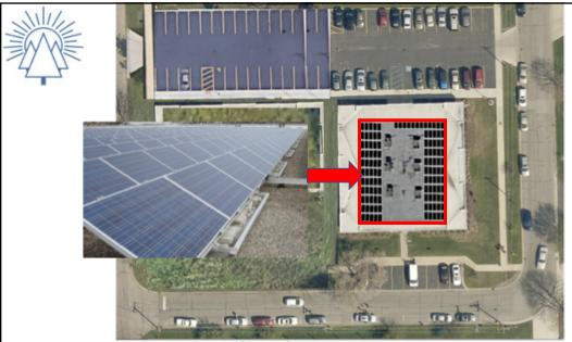
A 42kWh PV solar array will pay for itself in 12-14 years without subsidies...and save taxpayers over \$200,000 in electric bills over the first 25 years. PV panels have no moving parts or heavy electrical loads, so they last a long time. 30 year old arrays in Germany still operate at 80% efficiency!
