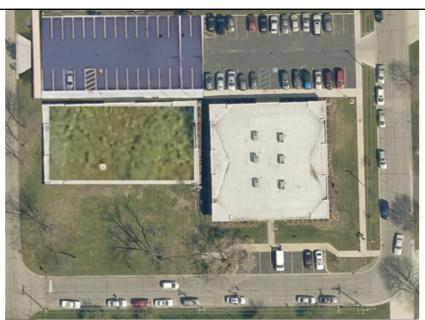
A green roof improves storm water management: it reduces runoff, improves water quality, conserves energy, mitigates the urban heat island, increases longevity of roofing membranes, reduces noise and air pollution, sequesters carbon, and provides habitat for wildlife.
